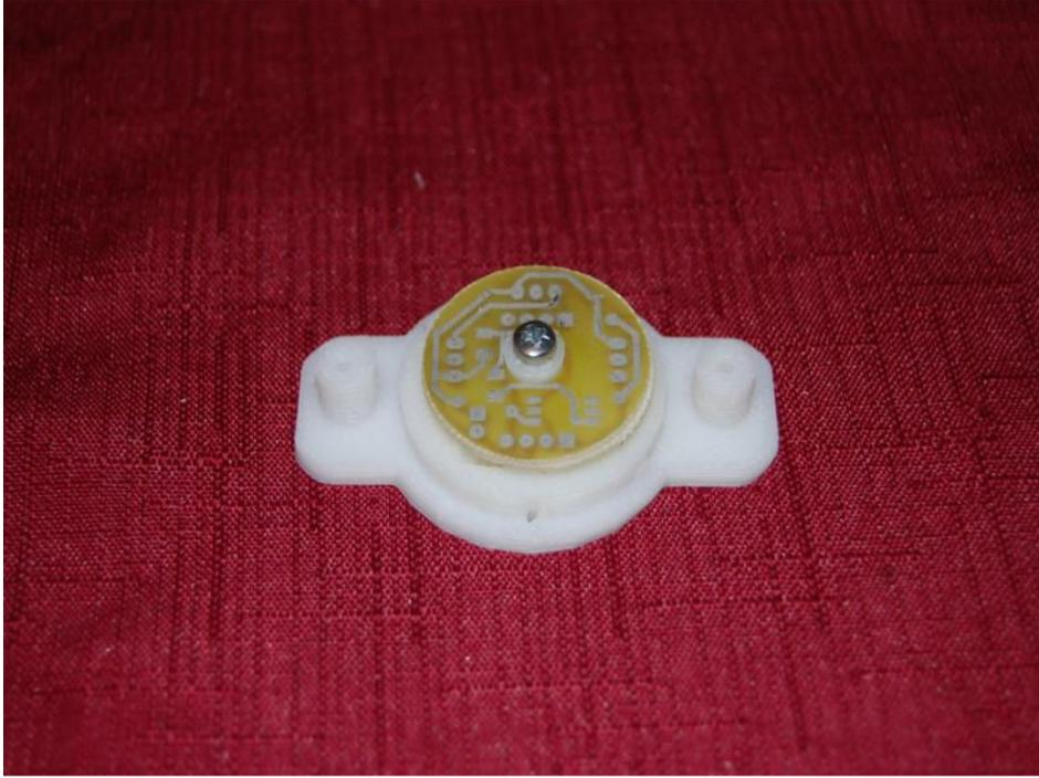
Place the sensor dome over the base and screw into place with 3 x #2 x 6.4mm self tap screws. Ensure that the screws are at right angles to the dome base as the dome may crack if the screws are not in line with the holes.
